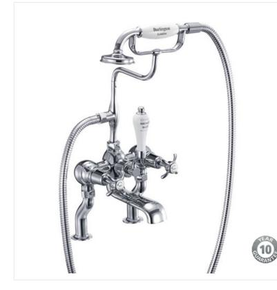
Anglesey bath shower mixer - deck mounted T8 Bath shower mixer (Including the standard cradle, 'S' adjuster, ceramic diverter, hose, ceramic telephone handset, excluding tap heads, bases and unions) T18 Deck mounting unions (for Bath Shower Mixer & Bath Filler, 3/4) T2 Anglesey tap handles (pair)
