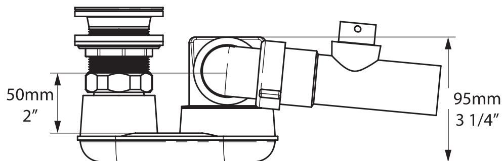
**Depth of Water Seal Conforms to BS EN 274-1**
