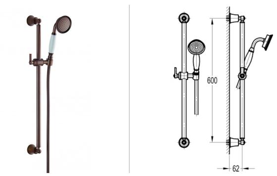
Dimensions are in millimetres except thread sizes which are BSP imperial.
