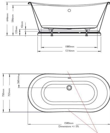
**IMPORTANT:** As the original Boat or Bateau baths were made, the rim on the long sides bend inwards by approx. 20mm in the middle, so there will be a gap between the centre of the bath and the wall
