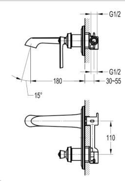
Dimensions are in millimetres except thread sizes which are BSP imperial.
