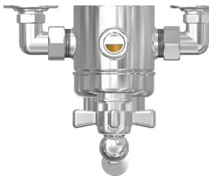
Supply connections are 15mm compression, and can be swivelled for top, bottom or through wall feed. Hot is on left, cold is on the right (viewed from front).
