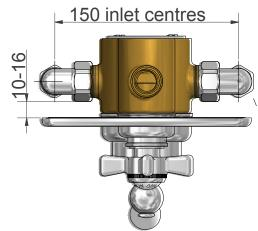
Supply connections are 15mm compression, and can be swivelled for top, bottom or horizontal feed. Hot is on left, cold is on the right (viewed from front).
