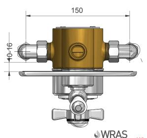
Supply connections are 15mm compression, and can be swivelled for top, bottom or horizontal feed. Hot is on left, cold is on the right (viewed from front).
