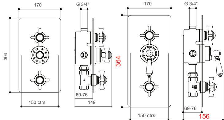
*When lever option is chosen for temperature (middle) handle use height sizes in red text*
