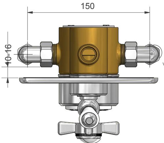
Supply connections are 15mm compression, and can be swivelled for top, bottom or horizontal feed. Hot is on left, cold is on the right (viewed from front).
