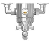
Supply connections are 15mm compression, and can be swivelled for top, bottom or through wall feed. Hot is on left, cold is on the right (viewed from front).
